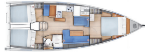
Version C Forward Owner's cabin, 2 aft cabins / 1 head Dressing + furniture with private sink in forward cabin, in option
